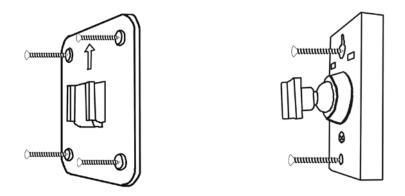
6. After the bracket is mounted, slide the transmitter down into place. The LED on the transmitter should be towards the top of the case to work properly.
